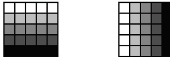
Figure 6. Horizontal and vertical linear gradient DCT basis vectors for the 5 \times 5 patch case.
