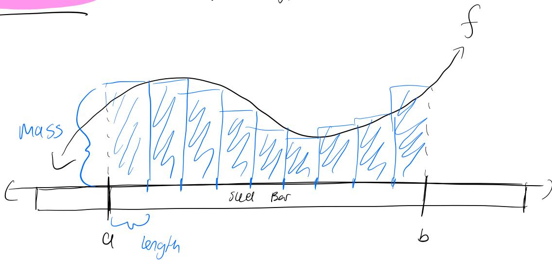
f - input is point on the rod and output is density at that point.
