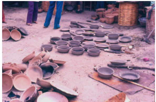
Figure 2.7 Pottery in the backyard of a potting household in Atzompa, Oaxaca, Mexico. The pots in the center are drying; those in the lower left corner have already been fired in the kiln (out of the photo, on the left). [Photo by author (1984).]
