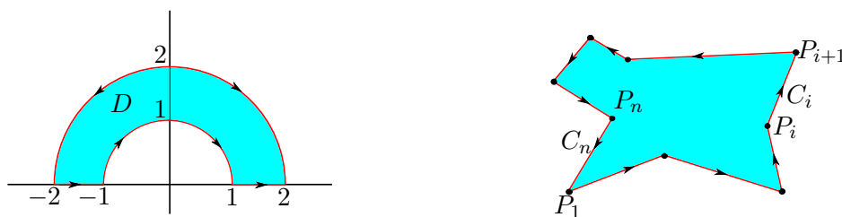
FIGURE 43.3. Left: The integration curve in the line integral discussed in Example 43.1. Right: A general polygon. Its area is evaluated in Example 43.3 by representing the area via a line integral.
